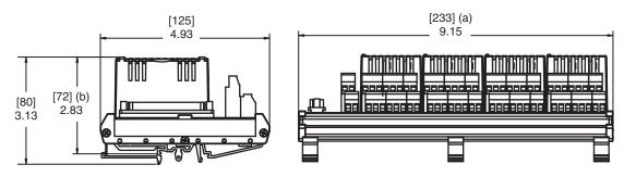
(a) Overall width – for determining DIN rail loading.
